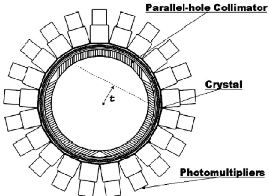
Fig. 1. Schematic illustration of CeraSPECT camera equipped with a three-segment parallel-hole collimator.
