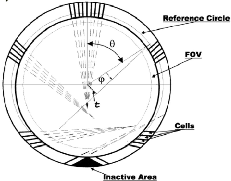
Fig. 2. Schematic illustration of the SensOgrade collimator. The collimator holes extend between two nonconcentric circles. All collimator holes are spaced equally on the reference circle.  $t$  is the transaxial distance, which is the distance between the center and the corresponding projection line,  $\theta$  is the angle between the vertical line and radial direction, and  $\phi$  is the angle between radial direction and projection line.
